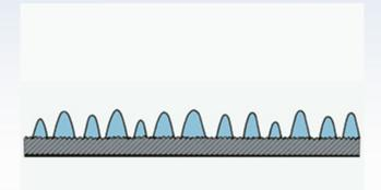
3. The particles cool and harden, welded to the surface, forming a series of "peaks" and "valleys" that provide a permanent base for the coatings.
