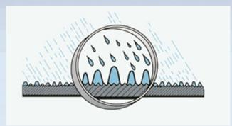
2. Then, the most important part: White-hot metal, including stainless steel, or ceramic particles are applied to the surface.
