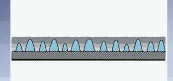
4. Several coats of tough nonsticks fill the "valleys" and cover the "peaks," locked permanently into place by the stainless steel "peaks."
