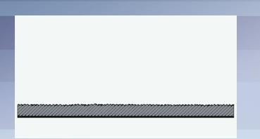
1. First, the surface of the pan is blasted with an abrasive to roughen it, so that other elements adhere better.
